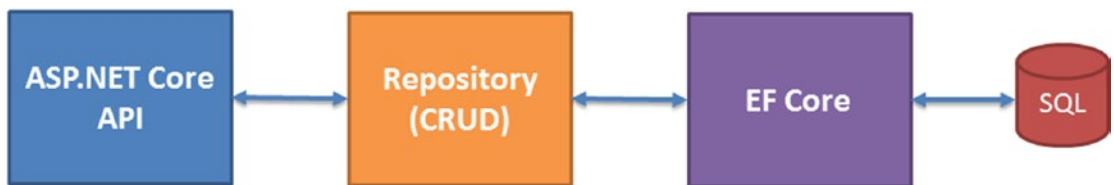
Figure 5-2. ASP.NET Core API uses the repository to perform CRUD operations
