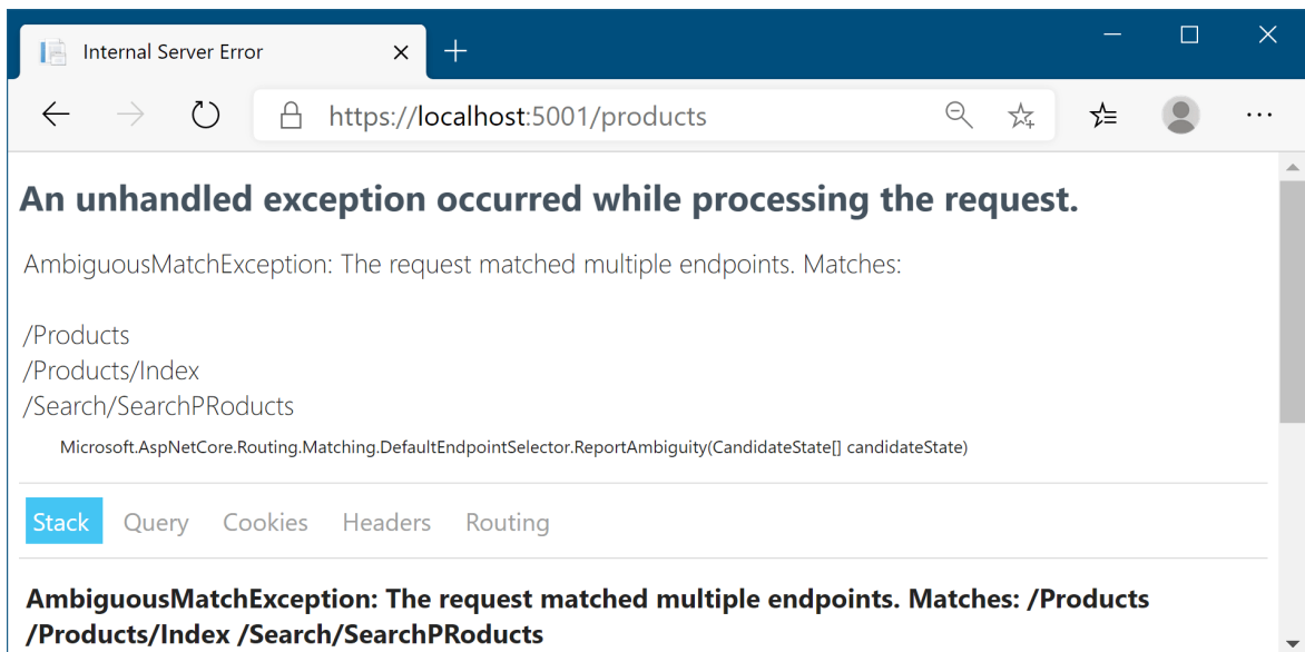
Figure 5.11 If multiple Razor Pages are registered with overlapping route templates, you'll get an exception at runtime when the router can't work out which one to select.
