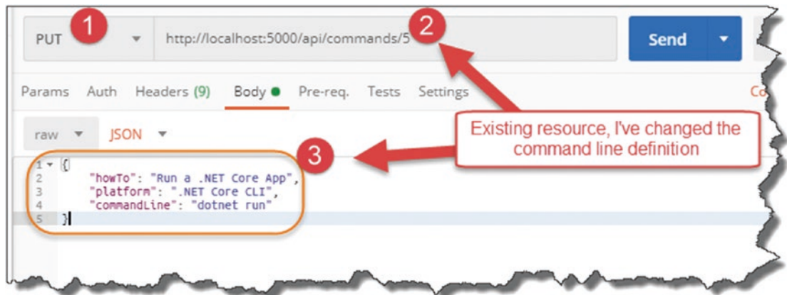
Figure 10-18. Testing the Put Action Result
