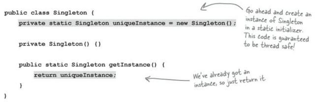
Using this approach, we rely on the JVM to create the unique instance of the Singleton when the class is loaded. The JVM guarantees that the instance will be created before any thread accesses the static uniqueInstance variable.
