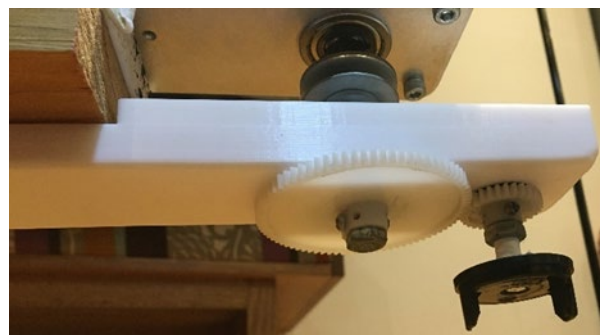
Figure 24: The gear multiplier and Beyblade launching end
