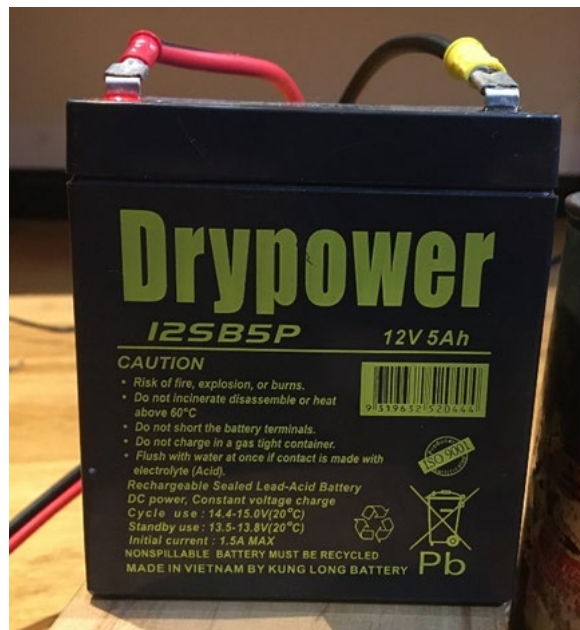
Figure 27: 12V Lead Battery
