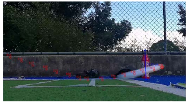
Figure 3: Snapshot of the tracker, process, where the blue bar indicates the calibration stick, and the red points represent the point mass location of the Frisbee at each frame
