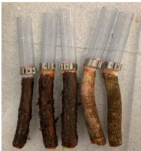
Figure 3: Angiosperm xylem filters with clear PVC and hose clamp attached to the branch.
