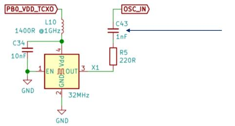
**C43**: When using NDK NT2016SA-32M-END4263A with an output of 0.8 V-pk-pk this capacitor must have **10 pF** of capacitance. See next page for more detail.
