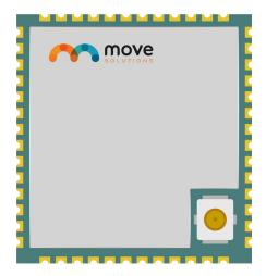
The MAMWLExx module is designed to be easily integrated to any PCB offering a U.Fl coaxial connector on the top of the package without the need for any developer to design a RF circuit for the antenna. If you wish to create your own antenna design, there is the chance to have the antenna directly on a 50 Ohm pin of the module.
