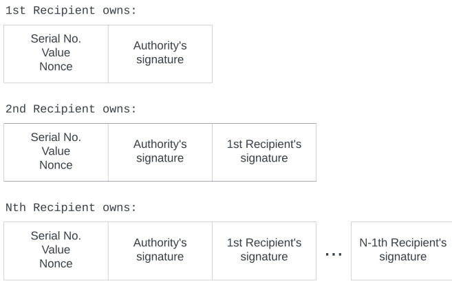
Fig. 1. Graphical representation of a token. Tokens represent monetary units of fixed value that store all their previous recipients until they are verified by an authority.
