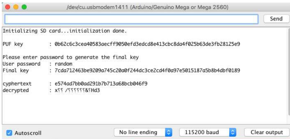
Figure 4.31: Screenshot of the bitcoin key storing experiment during decryption stage. The bitcoin key 'hahahahalalalala' is previously secured by using SRAM Cypress CY62256NLL 'D' and user's password 'qwertyuiop'. The bitcoin key cannot be reconstructed because user's password is wrong.
