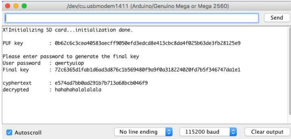
Figure 4.30: Screenshot of the bitcoin key storing experiment during decryption stage. The bitcoin key 'hahahahalalalala' is previously secured by using SRAM Cypress CY62256NLL 'D' and user's password 'qwertyuiop'. The bitcoin key can be reconstructed because user's password is correct.
