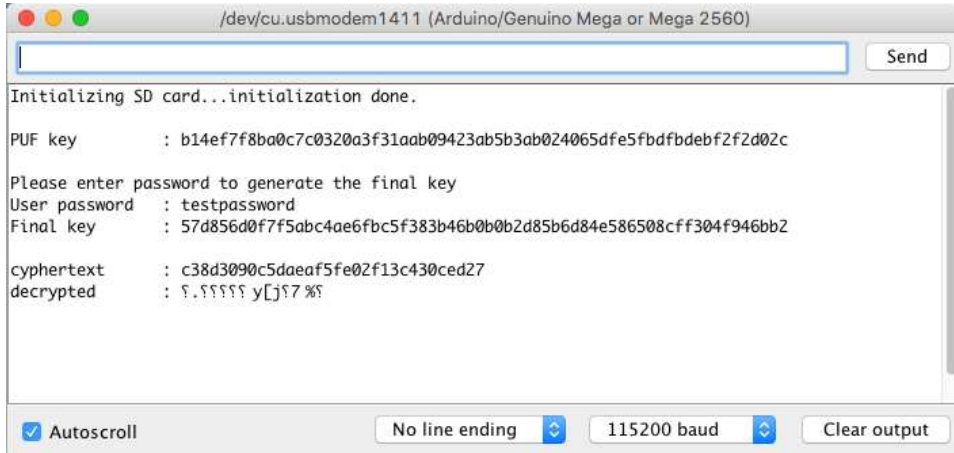
Figure 4.24: Screenshot of the bitcoin key storing experiment during decryption stage. The bitcoin key 'testpasswordtest' is previously secured by using SRAM Cypress CY62256NLL 'B' and user's password 'testpassword'. The bitcoin key cannot be reconstructed because the SRAM utilized for the decryption is SRAM Cypress CY62256NLL 'A'.
