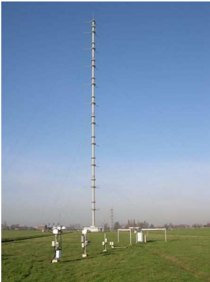
Figure 3.2. The Cabauw Experiment Site for Atmospheric Research (CESAR) used for the GABLS3 intercomparison study, showing the 213 m mast and radiation sensors (image courtesy of the BALTEX Office [93]).
