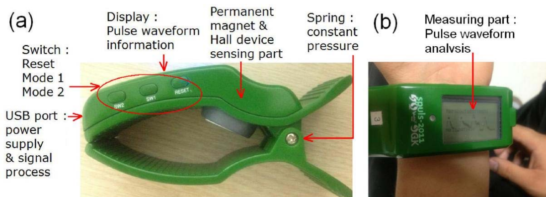
Figure 1. (a) The notation and function of several major parts and (b) the measurement process of acquisition pulse signals by a real clip-type pulsimeter.
