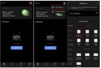
(1) Smart config mode: Press the reset button to switch device status until the device changes to Smart Config mode, and then add (please follow the instructions of the APP).
