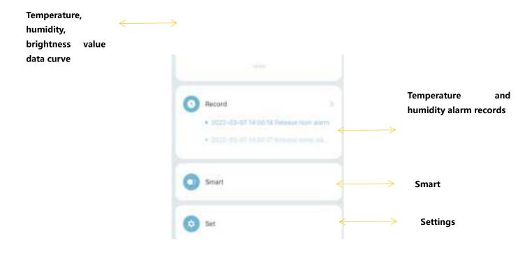
$\square$ . Temperature, humidity and luminance value data curve (temperature, humidity and luminance value data can be queried on the date of use)
