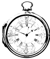
Figure 1.2 Harrison's H4. The first clock able to keep accurate time at sea, enabling determination of longitude.
