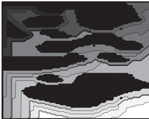
Figure H.9 A plot of linklength values from the start (upper left corner) node where colored pixels correspond to link lengths of paths defined by the depth-first search. The lighter the pixel the greater the linklengths in the graph; black pixels correspond to obstacles.
