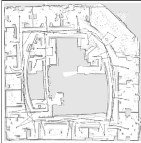
Figure 9.20 Map obtained by applying a scan-matching approach to the same data used in figure 9.19.
