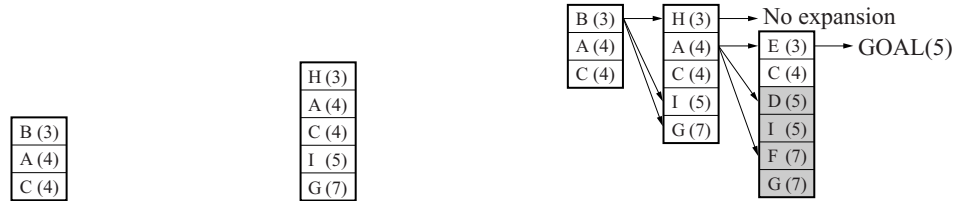
Figure H.12 (Left) Priority queue after the start is expanded. (Middle) Priority queue after the second node, B, is expanded. (Right) Three iterations of the priority queue are displayed. Each arrow points from the expanded node to the nodes that were added in each step. Since node H had no unvisited adjacent cells, its arrow points to nothing. The middle queue corresponds to two actions. Node E points to the goal which provides the first candidate path to the goal. Note that nodes D, I, F, and G are shaded out because they were discarded.
