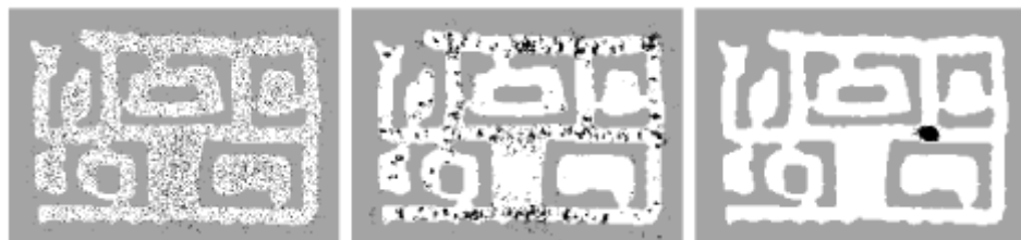
Figure 9.7 Global localization using a particle filter with 10,000 samples. The left image shows the initial distribution. The middle image shows the distribution after incorporating ten ultrasound beams. The right image shows a typical situation (here after 65 steps) when the location of the robot has been identified.
