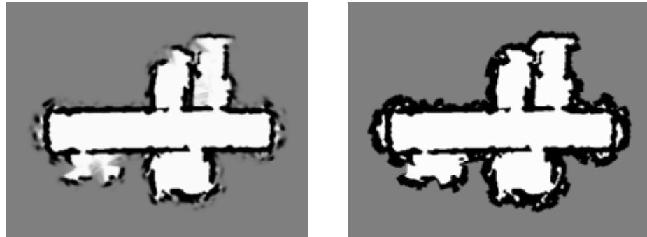
Figure 9.18 Occupancy probability map for the corridor of the Autonomous Intelligent Systems Lab at the University of Freiburg (left) and the corresponding maximum-likelihood map (right).
