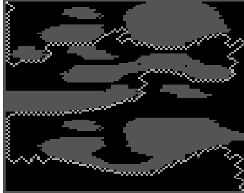
Figure H.8 White pixels denote the path that was determined with depth-first search.
