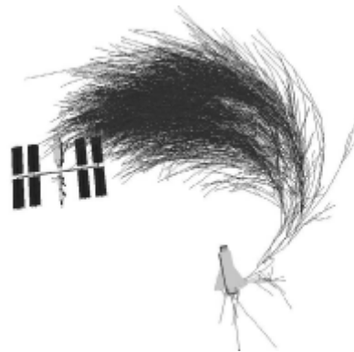
Figure 7.11 Tree generated by a tree-based motion planner for docking a space shuttle at the space station. (From Phillips and Kavraki [350].)
