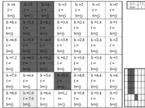
Figure H.17 Start node is put on priority queue, displayed in upper right.
