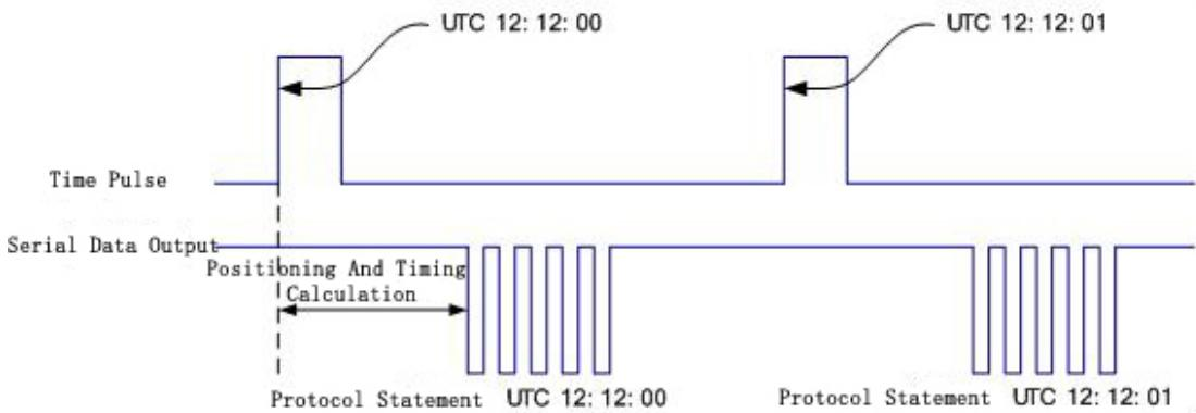
AT3340 dual mode receiver module board support for the configuration of PPS pulse output mode. Configurable items include: pulse interval, pulse width, pulse on and off, pulse polarity, time reference, time information source and pulse delay. The configuration statement is shown in the following table:
