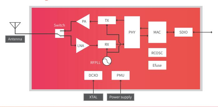
The WLAN subsystem includes a single-band 2.4G RF transceiver (RX and TX), PA and LNA including RF switch, RFPLL, PMU, OFDM/CCK PHY and MAC processor, that keep data communications with host using SDIO 2.0. This application has industry leading low cost BOM to simplify product development.
