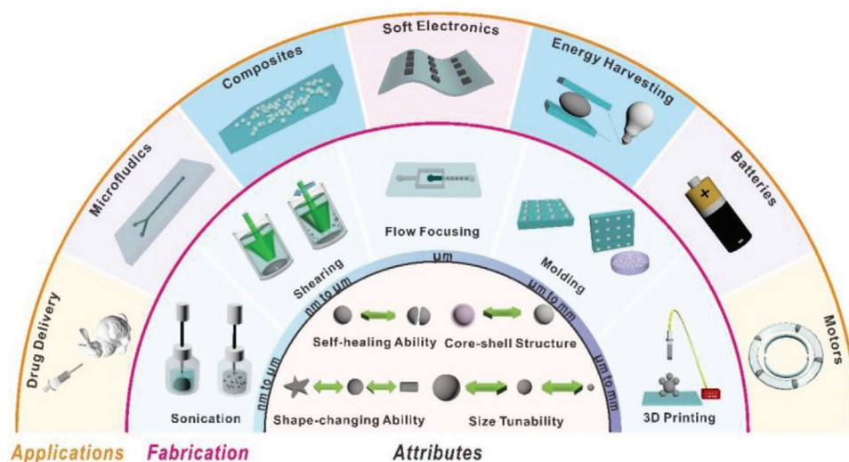
Figure 2. Attributes, fabrication, and applications of liquid metal particles. 1) The inner semi-circle illustrates the attributes of liquid metal particles; 2) the middle annulus describes methods to fabricate liquid metal particles with different sizes; 3) the outer annulus presents several applications of liquid metal particles.
