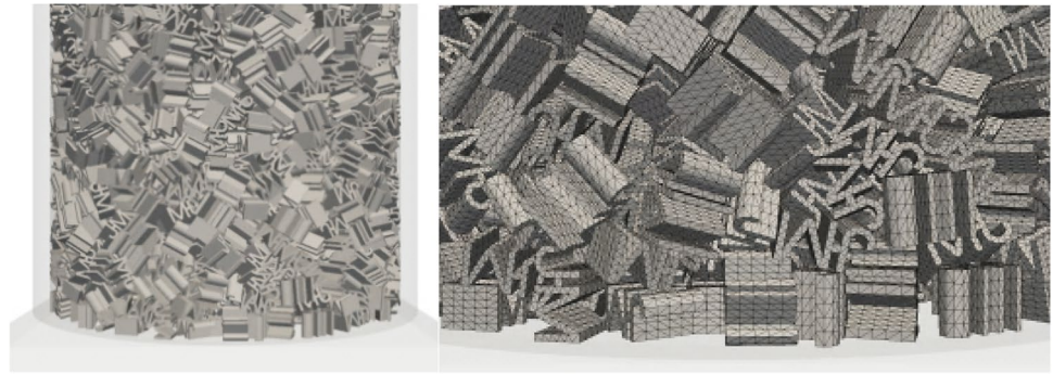
Fig. 5 Packing structure at bottom of a cylindrical container simulated with FDEM in Solidity for ‘lettering pellets’ made from CAD file extrusion; to illustrate packing of a highly concave-shaped particle, and close-ups showing the tetrahedral mesh elements
