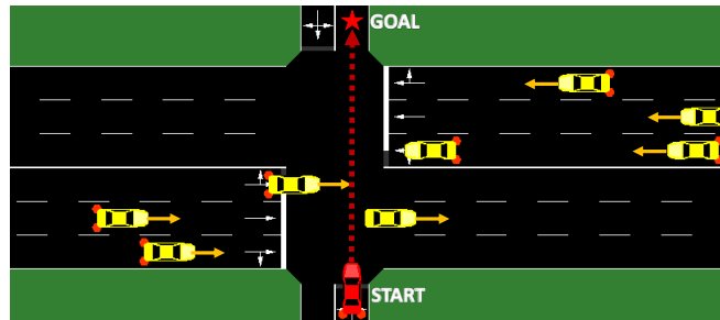
Fig. 1: Crossing a busy intersection. Red car is the autonomous vehicle and yellow cars are oncoming traffic. The objective is to determine the acceleration profile along the path.
