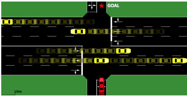
Fig. 6: DQN Time-to-Go predicts the opening and begins accelerating in anticipation of the clear path. TTC would have waited until all cars were clear, missing the opportunity.
