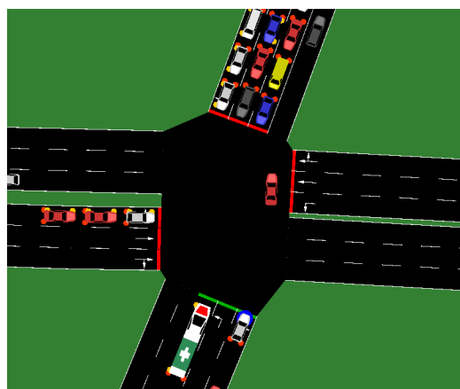
(a) Emergency vehicle receives priority at intersection
