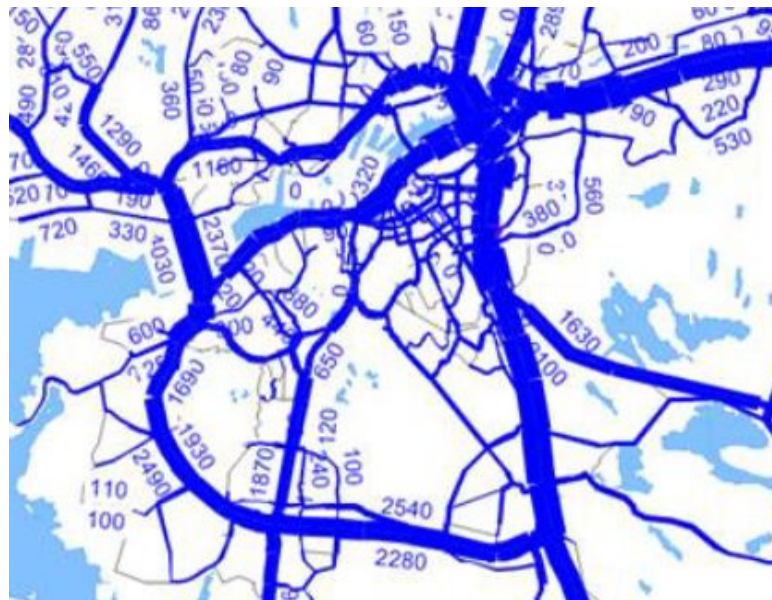
Figure 1.5: The inflows and outflows from a VISUM traffic model for rush hour between 16:00 to 17:00 on and around the Drive Me route.
