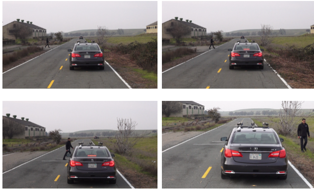
Fig. 8. Steps for stopping for a pedestrian. a) A pedestrian is detected that is currently not on the road. b) Pedestrian enters the road, triggering the AD vehicle goes into stop state. c) vehicle remains in STOP state until the pedestrian is cleared. d) vehicle resumes to the GO state after pedestrian leaves the road boundary.
