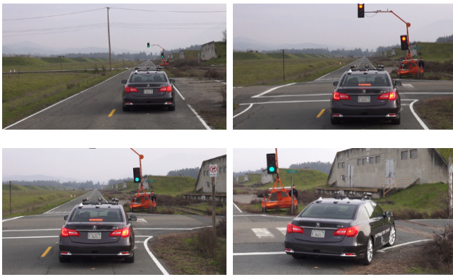
Fig. 5. Steps for handling a signalized right turn. a) Green light is detected from a distance of approximately 80m. Anticipating there is an upcoming right turn, vehicle goes into STOP state. b) The light turns to red, which is correctly recognized, and the AD vehicle comes to a full stop. c) Light turns green, state and the AD vehicle is cleared to continue. Absent cross-traffic, the vehicles resumes to the GO state. d) AD vehicle makes the right turn.
