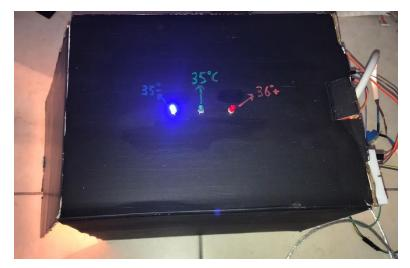
Here, the temperature inside the box is below desired level. The lightbulb is turned On by the program an it will stay that way until required temperature inside the box has been reached.
