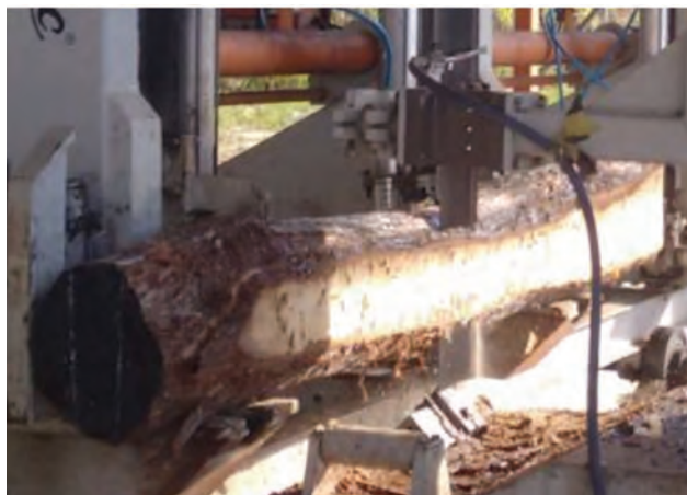
Figure 2. Primary sawmilling of logs using a vertical bandsaw, with 1.20 m diameter wheels and advance/feeding by a semi-automatic feeder.
