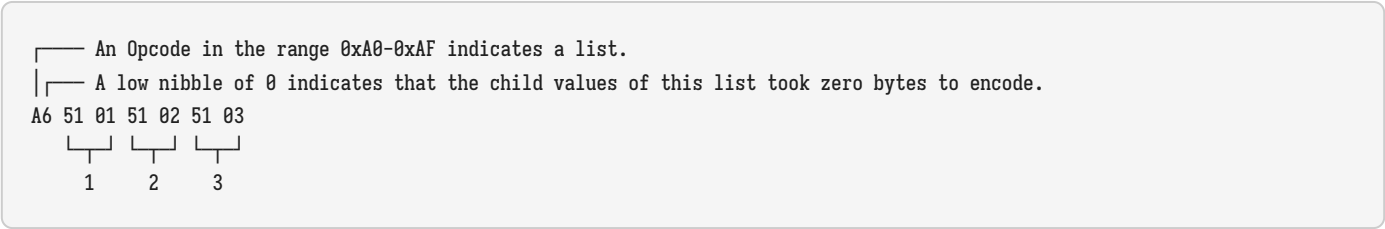
Figure 65: Length-prefixed encoding of [1, 2, 3]
