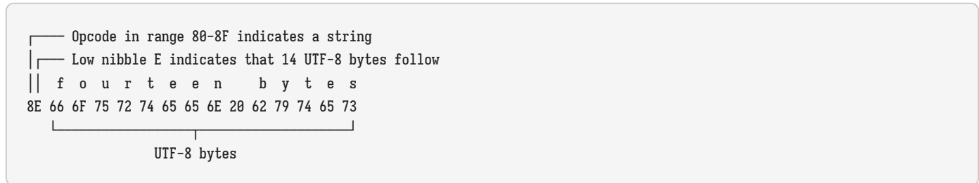
Figure 53: Encoding of a 14-byte string
