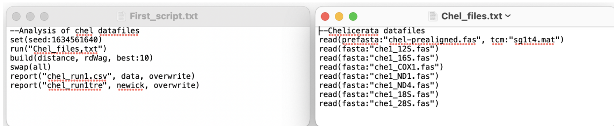
Figure 1.1: PhyG scripts. The headers in the scripts are comments, leading with ‘ -- ’, which is ignored by PhyG . This first script “ First_script.pg ” includes a reference to the second script “ Chel_files.txt ”, which includes a group of data files to be read by the program.
