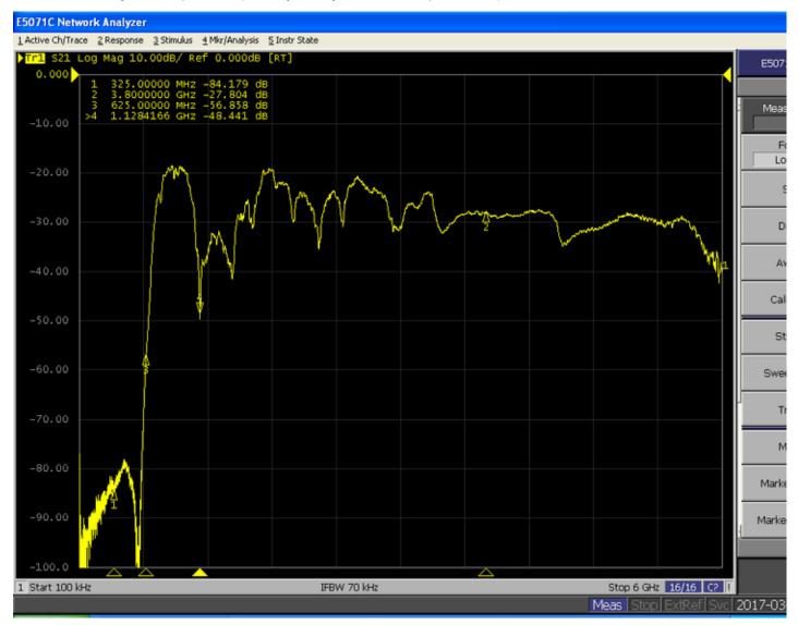
You can see thing over 625 MHz, the antenna has pretty good performance, with the exception of a tight notch at 1.12 GHz. This means unless you are really close to an FM broadcast station, you will not be able to receive FM with this antenna. (it has been done, and it does work - it just limits the distance between you and the antenna. Remember that most terrestrial FM broadcast stations are 10,000 to 20,000 watts).
