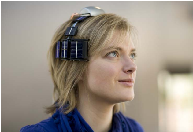
Figure 8. Two-channel wireless EEG system with hybrid energy scavenger.
