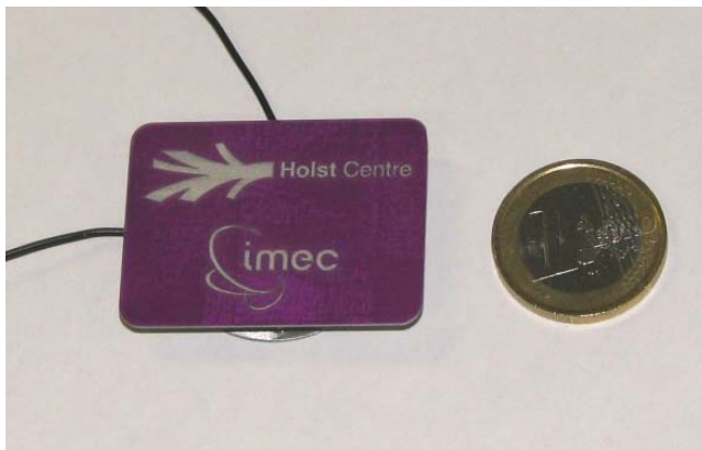
Figure 10. Thermoelectric module of the shirt compared with 1 Euro coin.
