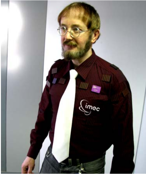
Figure 9. Body-powered wireless electrocardiography shirt.
