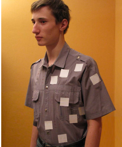
Figure 1. The shirt used for measurements of the thermal resistance of human body.
