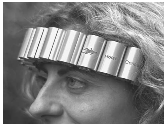
Fig. 4. Two-channel wireless electroencephalography system with a 2.5-mW thermoelectric generator.
