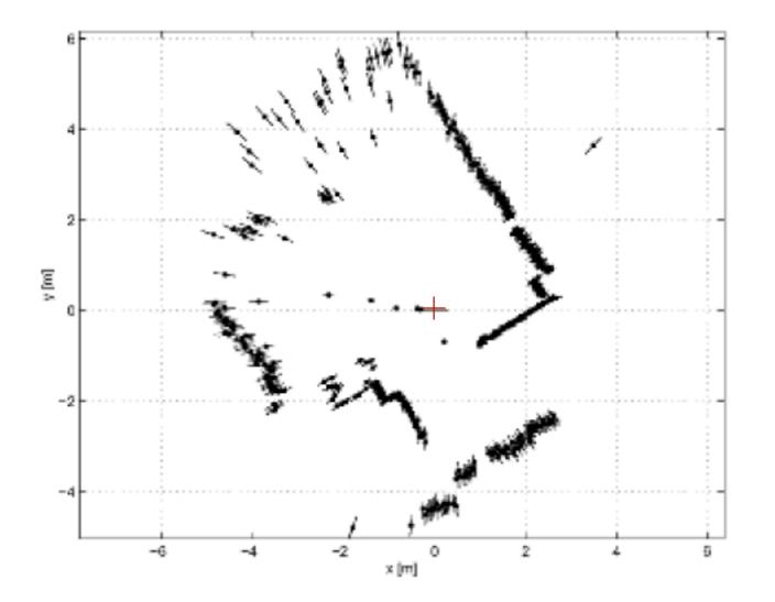
use the whole scan as output vector: its components are the range readings in all available directions  the innovation is then computed as the difference between the actual scan and the predicted scan
