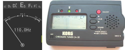
Fig. 1. Examples of chromatic tuners: gStrings on Android (left) and Korg CA-30 (right).
