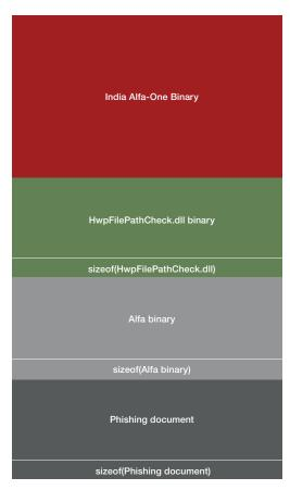
Figure 2-1: Payload File Stacking within IndiaAlfa-One Samples
