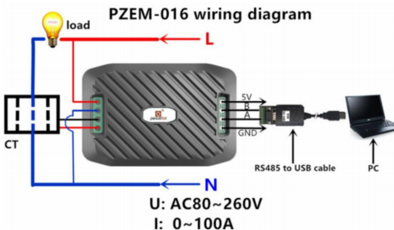
Picture 4.2 PZEM-016 wiring diagram
