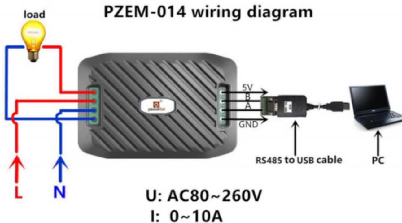
Picture 4.1 PZEM-014 wiring diagram
