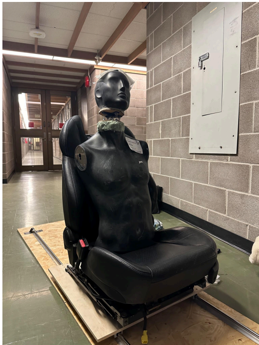
Figure E.1: Final Sled Assembly
