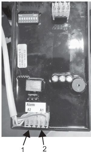
Fig. 4: Cable connection at the control unit
