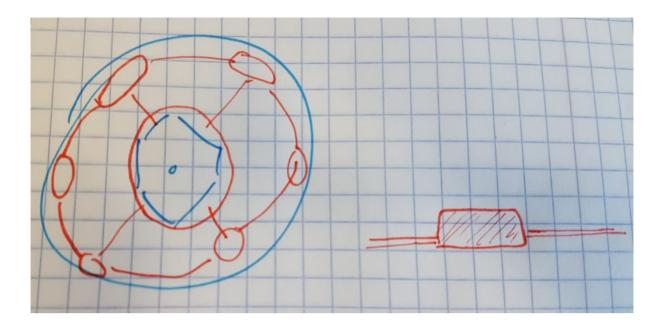
The reason that the cape should not simply be a cylinder is because this will block too much of the IR signal, and likely not provide any discrimination between sensors mounted at different angles; and if it does, it still might not be relevant for bee-generated signals.
