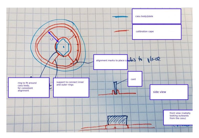
Here, the outer ring of the cape is a guide to support inserting a piece of card; this will allow testing of various different sizes of occlusion - just by cutting different width/height of card - to identify the size of occlusion so that it is relevant, i.e. in the sensitive range.
