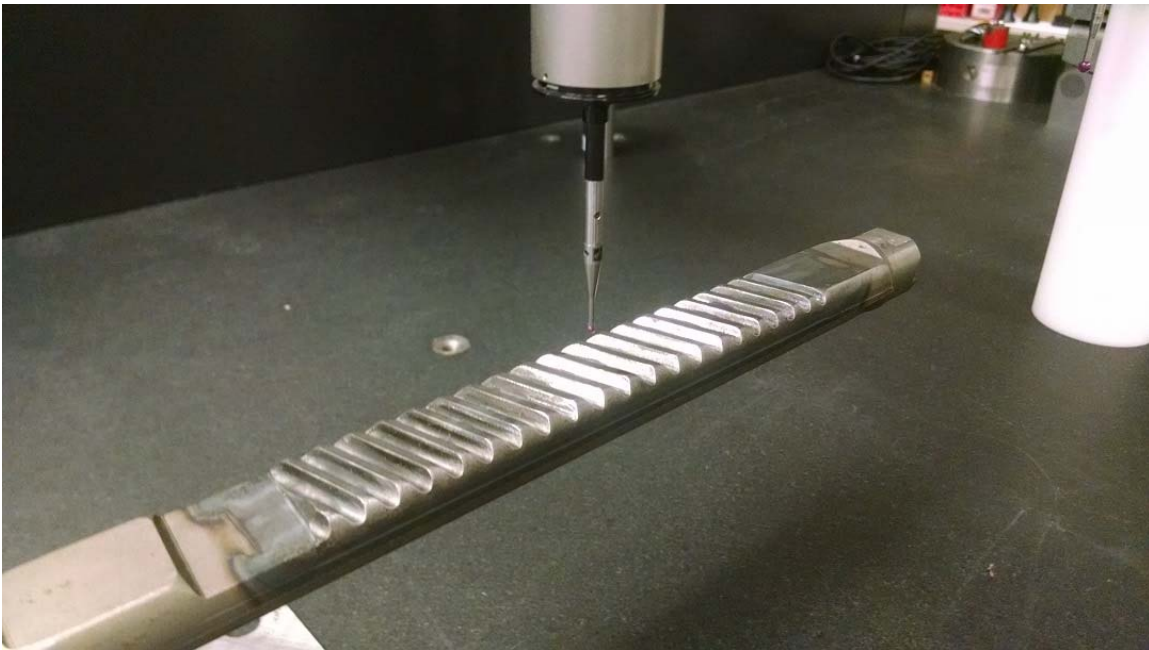
CMM Measurement of Rack Tooth Height to Rack Centerline
