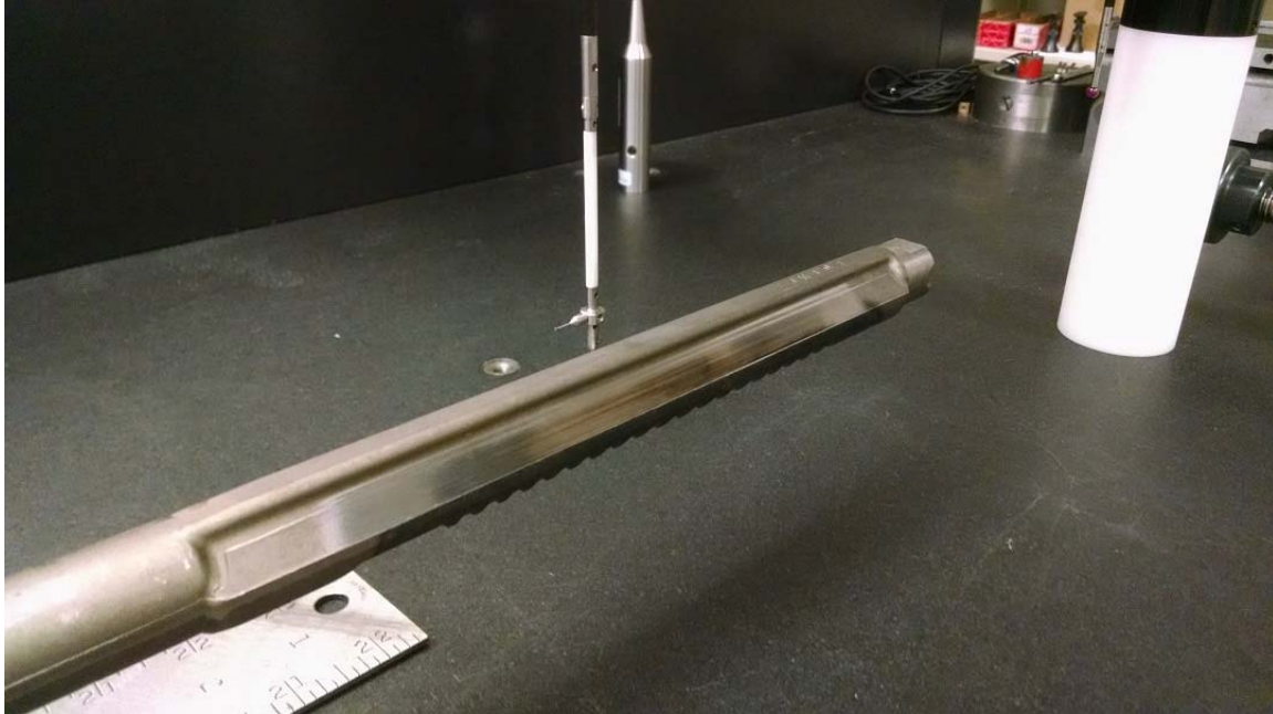
CMM Profile Trace of Y-Form Rack Bar
