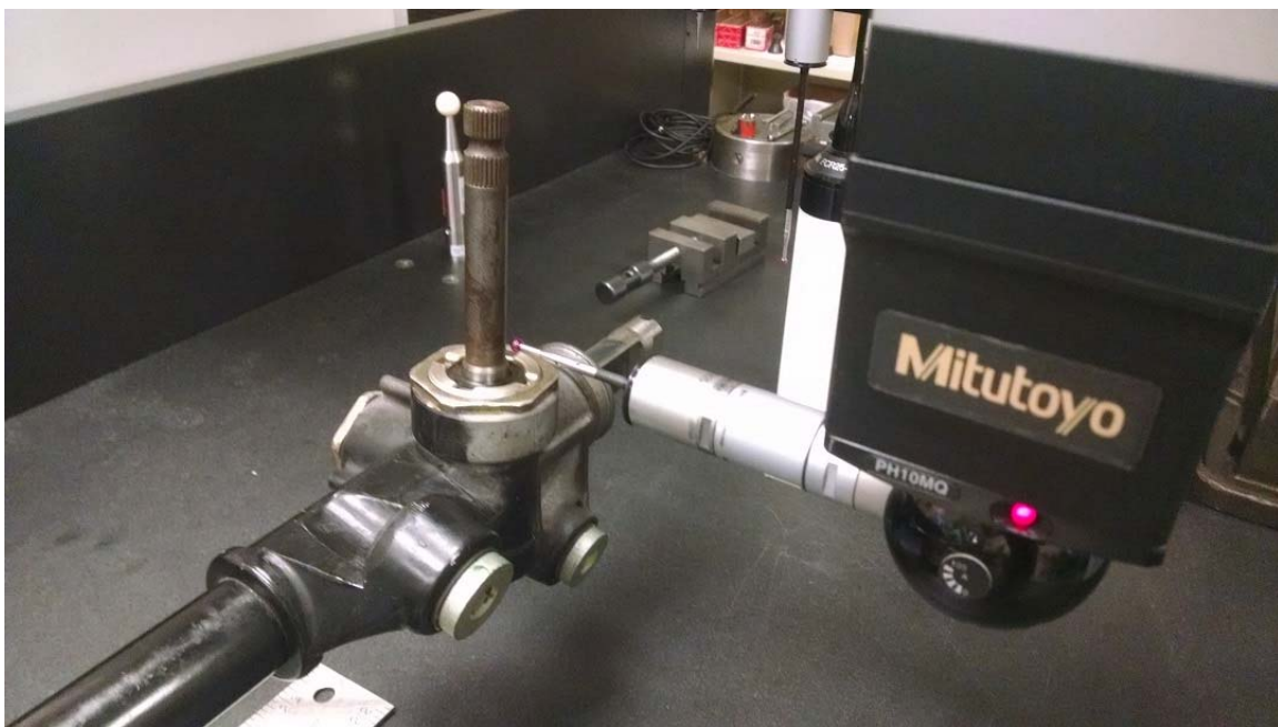
CMM Probe Measuring Point on Pinion Shaft
