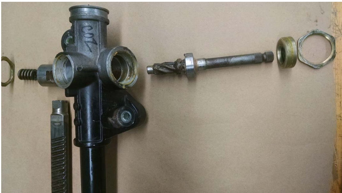
Disassembled Steering Gear – Pinion with Upper Bearing, Pinion Retaining Screw, and Nut
