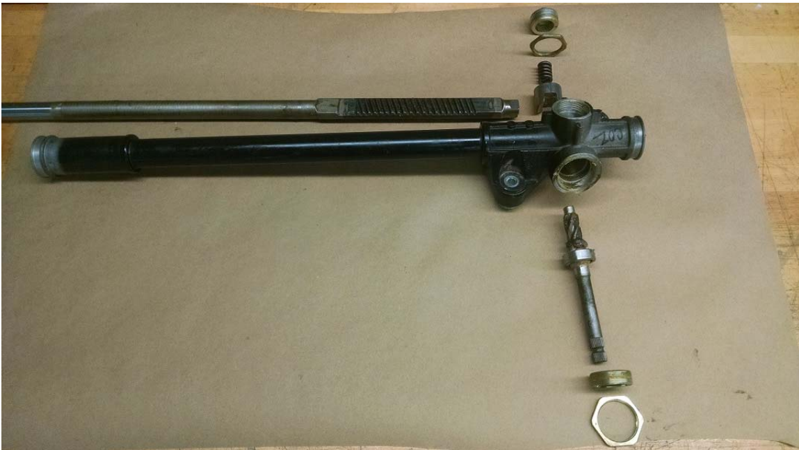
Disassembled Steering Gear – Rack, Pinion, and Yoke Assembly Removed
