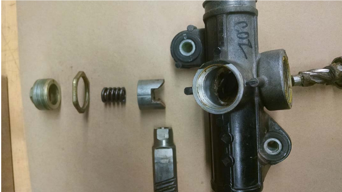
Disassembled Steering Gear – Yoke Screw, Yoke Nut, Yoke Spring, and Yoke
