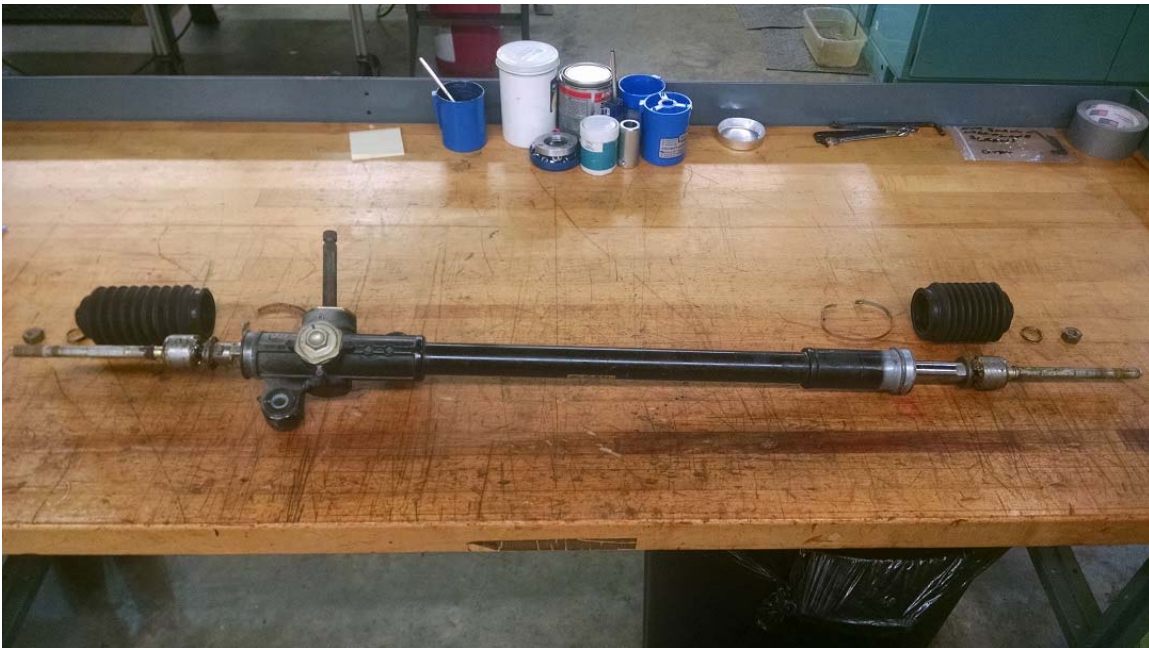
Steering Gear with Bellows Removed
