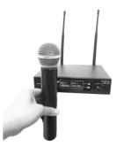
4. Connect receiver to mixer or amplifier. Make sure audio levels on the mixer are muted or off. For PA System, use the 1/4" AF output (line level unbalanced, 4b). For all other applications use the XLR output (mic level, 4a)
