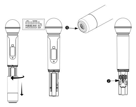
1. Microphone Battery Installation
