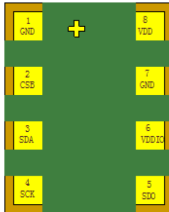
Figure 5: Layout pin configuration SPA06-003 (Bottom View)
