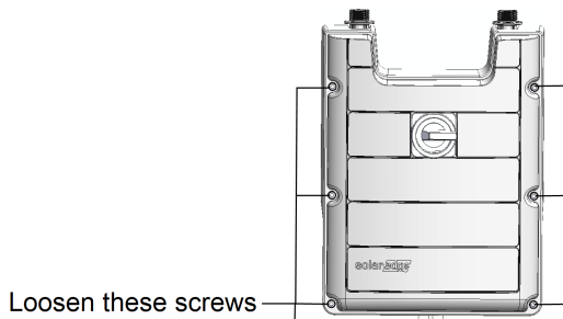
Figure 10: Opening the StorEdge Connection Unit cover
