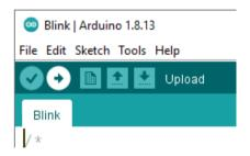
If the upload does not work at the first attempt, it may help to press the "Boot-Button" on the module during the upload. Please use a USB 2.0 certified cable for programming.
