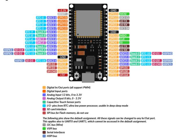
For detailed pinout decription and I/O capabilities please refer to the datasheet which can be found on the following link.
