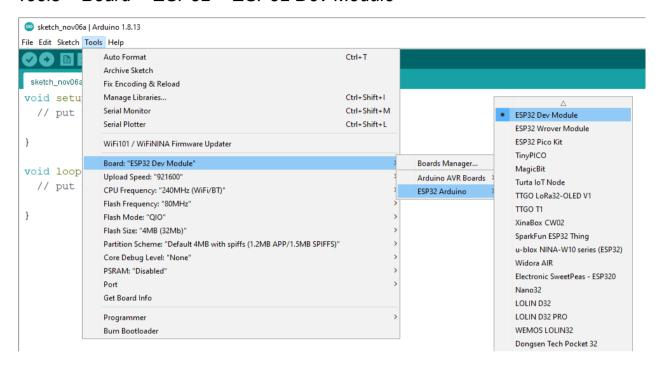
To upload the sketch code to the ESP32 board, first select port on which you connected the board. Go to: *Tools > Port > {port name}0*
