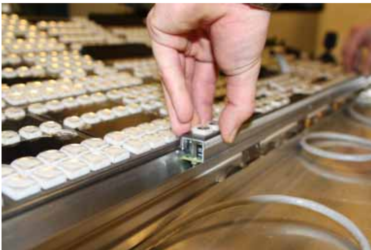
Aligning the System Bar for Replacement
