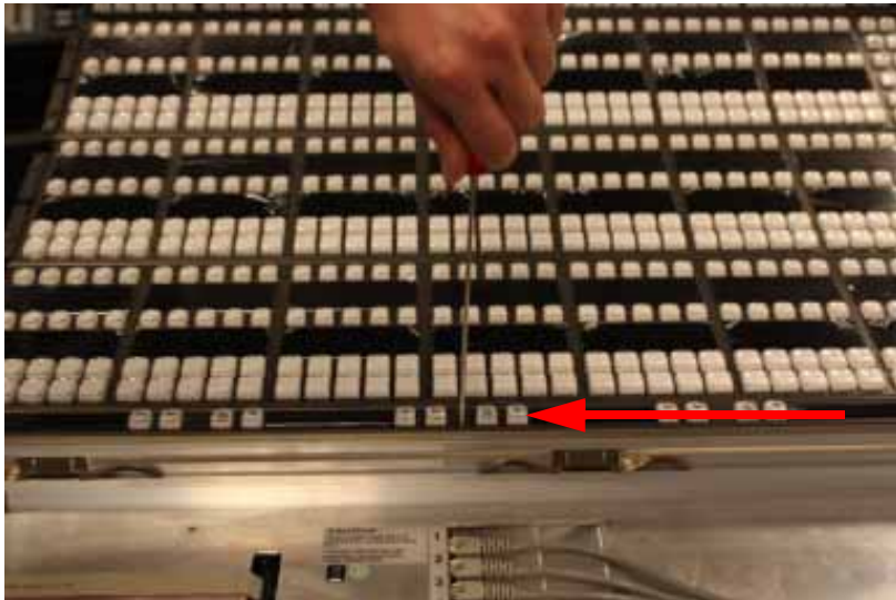
Unscrewing the System Bar
