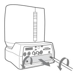
2 Insert an optional Interface Board into the card slot. Align both ends of the Interface Board with the sliders inside the slot, then insert the board securely as far as it will go.
