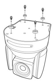
Attach the ceiling bracket (A) to the bottom of the camera using the supplied four screws (⊕M3 × 8). Position the O hole for screwing on the ceiling bracket (A) to the front of the camera as illustrated, align the screw holes on the ceiling bracket with those on the bottom of the camera, then attach the bracket to the camera.
