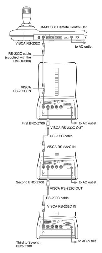
You can connect the camera to a computer equipped with the VISCA RS-232C connector instead of the connection to the RM-BR300 Remote Control Unit.
