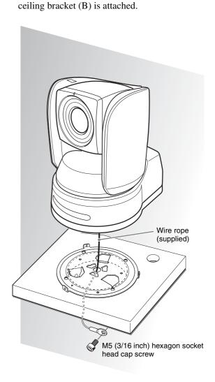
Insert the protrusions on the ceiling bracket (A) into the spaces prepared in the ceiling bracket (B) with the O hole in the front of the ceiling bracket (A) aligned with the  $\diamondsuit$  hole on the ceiling bracket (B), and temporarily attach them by turning the ceiling bracket (A) with the camera counterclockwise.
