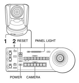
1 Connect the camera to an AC outlet using the supplied AC power adaptor and power cord. The power is turned on and the POWER lamp lights.
