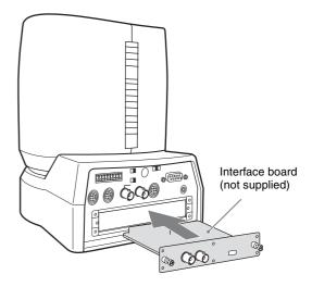
**3** Tighten the two screws on the Interface Board.
