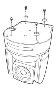
Attach the ceiling bracket (A) to the bottom of the camera using the supplied four screws (⊕M3 × 8). Position the ○ hole for screwing on the ceiling bracket (A) to the front of the camera as illustrated, align the screw holes on the ceiling bracket with those on the bottom of the camera, then attach the bracket to the camera.
