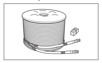
This is a 2-core multi-mode optical fiber cable of 100 m (328 feet) long.
