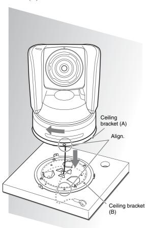
Secure the ceiling brackets (A) and (B) using the supplied three screws ( $\oplus M3 \times 8$ ).
