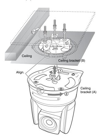
8 Secure the ceiling brackets (A) and (B) using the supplied three screws  $(\oplus M3 \times 8)$ .
