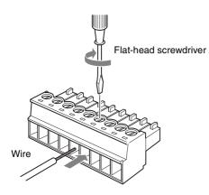
Insert the VISCA RS-422 connector plug into the VISCA RS-422 connector.
