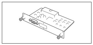
The board allows output of a signal conforming to the VESA standards (VGA, XGA or WXGA).
