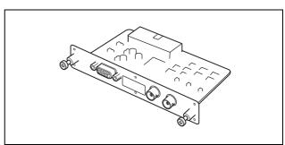
The board allows output of an analog video signal such as the composite video, S video, component video and RGB signals, or a down-converted SD-SDI signal. An audio signal of the SD-SDI signal is not output from the board.
