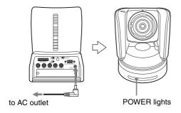
1 Connect the camera to an AC outlet using the supplied AC power adaptor and power cord. The power is turned on and the POWER lamp lights.
