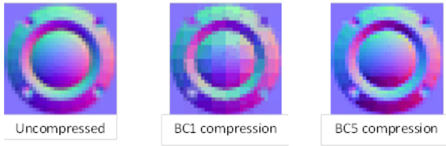
Figure 10. Normal map compression. (Source: ATI 3Dc White Paper (29))
