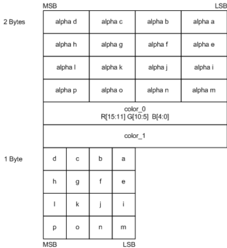
Figure 7. BC2 block layout. (Source: Programming Guide for Direct3D 10 (27))
