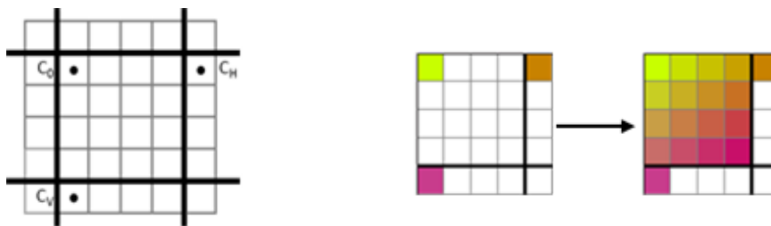
Figure 25. Base color position for ETC2-Planar block and decompression example.
