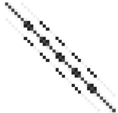
Figure 3.11: PETSc can show the matrix structure too. The actual graphic is in color, but here the two dark shades show positive and negative entries while the light shade shows allocated locations which are zero.
