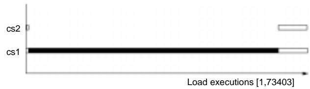
Figure 8. Value trace of load d4531 in m88ksim. This load restores the return address register. Since the load returns only two unique values, addunsigned is called from only two call sites during this run.
