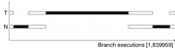
Figure 4. Execution trace of b35 on the input scene1 . We use shading to distinguish contiguous segments of taken (or not-taken) executions from those segments that have an interleaving of taken and not-taken executions. For example, between executions 183272 and 595513, inclusive, b35 is only taken.
