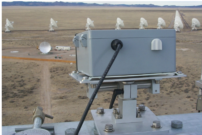
Figure 8: Holography system hardware. Signal feed side of the frontend (top); reference feed side of the frontend (middle); and transmitter.
