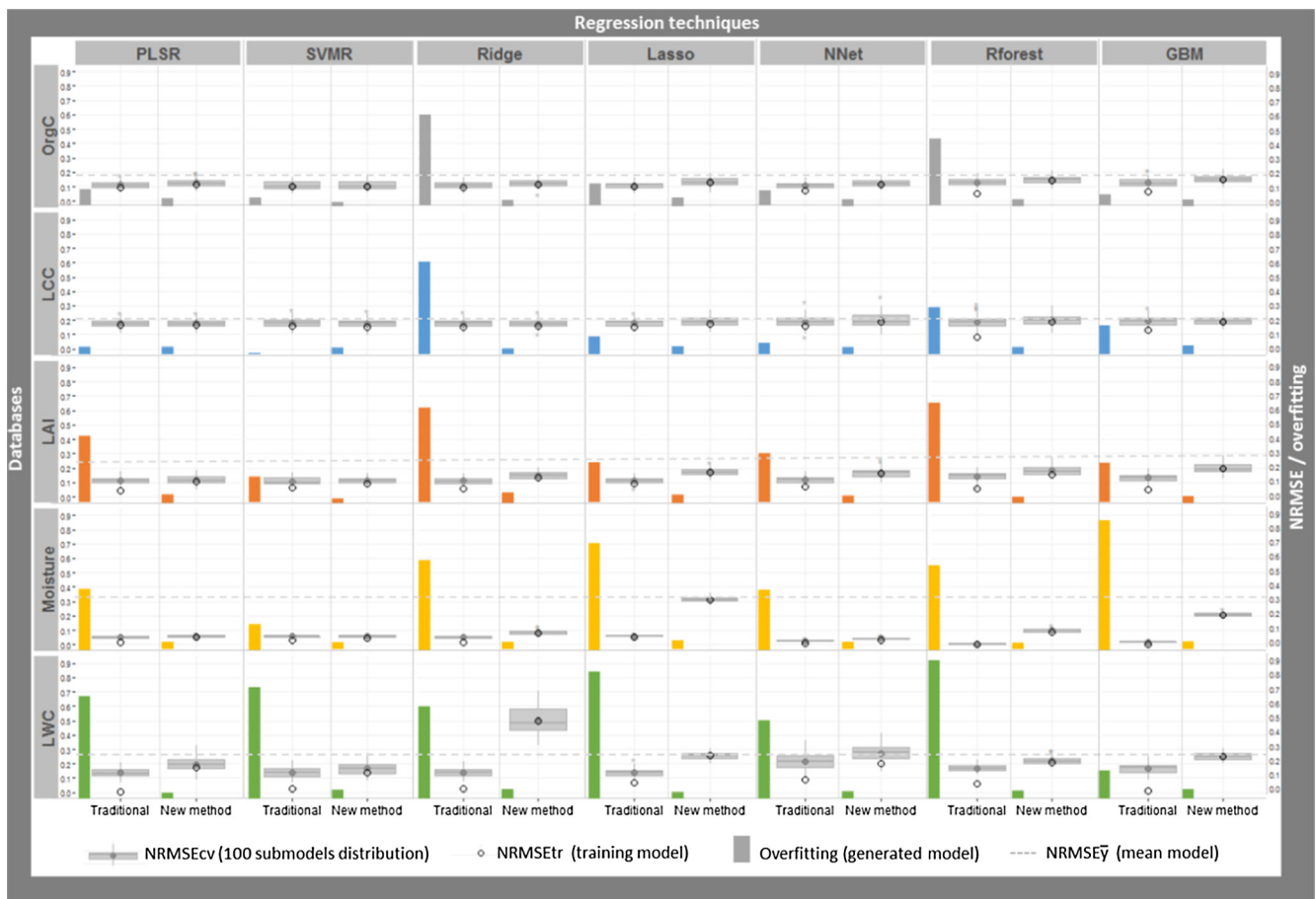
Fig. 5. Boxplots of the NRMSE distribution from 100 cross-validated models fitted on the original bands with a model complexity selected by the traditional and NOIS method. The bars represent the naïve overfitting index of the model complexity selected. The circles indicate the NRMSE tr using all the observations.
