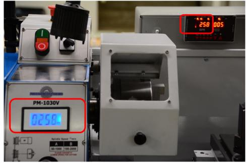
They agree perfectly, so that indicates that I have all of that section wired correctly and that the encoder settings in configuration.h in the code are correct.
