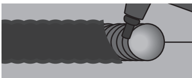
PARTIALLY CHIPPED AWAY TO SHOW WELD
